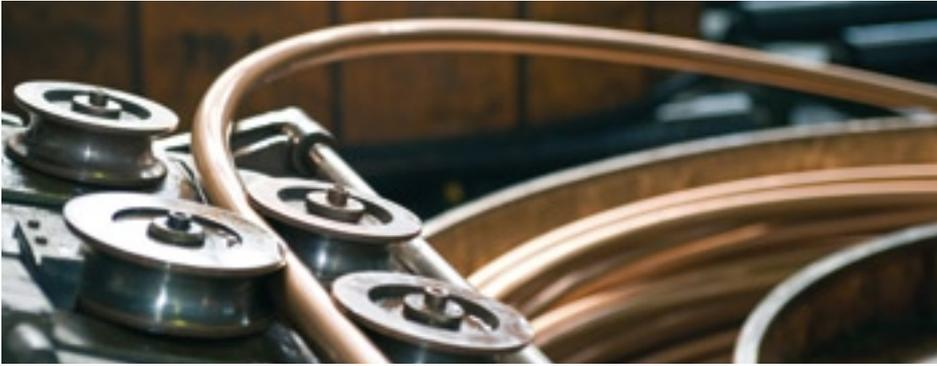
The starting products are refined copper billets delivered from continuous casting plants. These are heated to 950 °C and processed into hollows for further processing by hot pressing or hot skew rolling. Reciprocating rolls then perform the subsequent cold forming. Hard, half-hard and soft copper tubes are produced for domestic plumbing in multi-stage cold-drawing processes.
